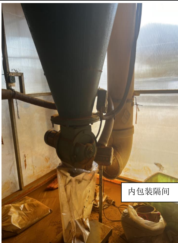
粉碎、包装粉尘：内包装隔间+集气罩+集中抽气
