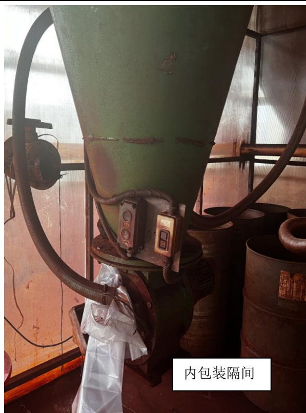
粉碎、包装粉尘：内包装隔间+集气罩+集中抽气
